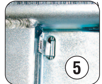
Underside Shown, looking up "Emergency Brake Set"
